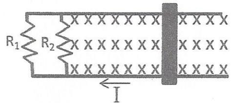
What is the direction of the moving bar (left or right) and what is the current induced in the circuit?
