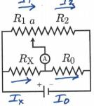
The contact position *a* is varied until there is **no current** flowing through the ammeter (A). What is the resistance of  $R_X$  as a function of  $R_0$ , *a*,
