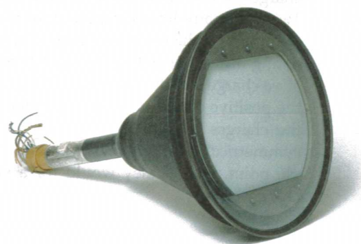
A cathode-ray-tube display used for color television. The beams of electrons from the electron gun on the left activate phosphors on the screen at the right, giving rise to bright spots whose colors depend on the relative intensity of each beam. Electric fields between deflection plates in the gun (or magnetic fields from coils surrounding the gun) deflect the beams. The beams sweep across the screen in a horizontal line, are deflected downward, then sweep across again. The entire screen is covered in this way 30 times per second. (Science & Society Picture Library/Contributor/Getty Images.)
